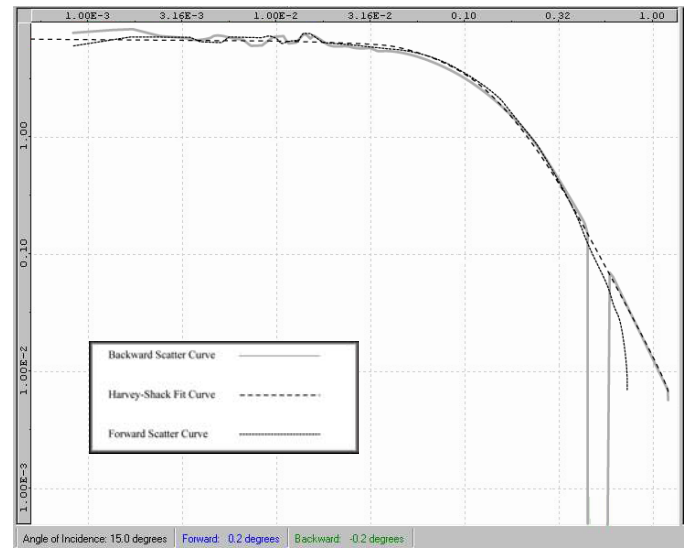
Figure 7. BRDF data and Harvey-Shack fit for HLA painted sample. 15 degree angle of incidence [1]
